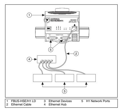
Figure 1-1 shows an FBUS-HSE/H1 LD connected to an Ethernet network.
